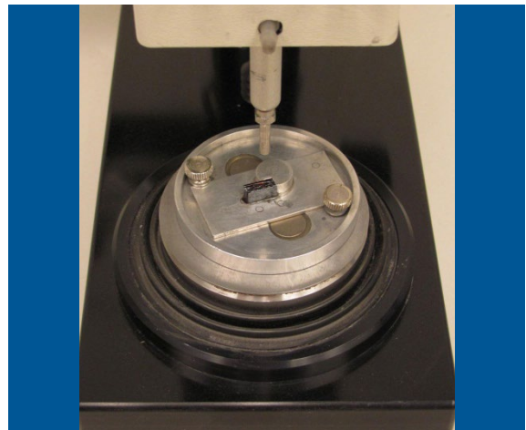
Figure 4. Center the cutting diameter over the third and fourth pieces in the silicon stack.
