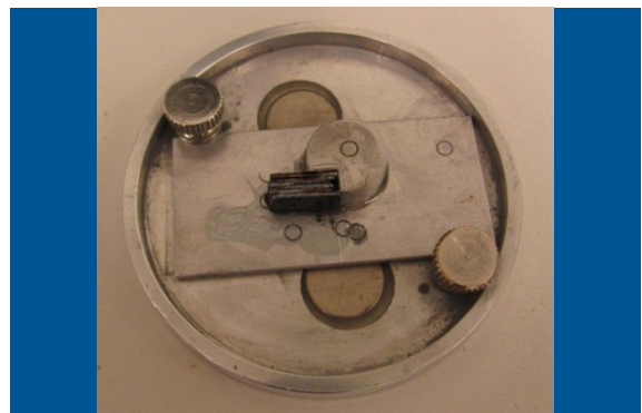
Figure 3. Aluminum plate and silicon stack mounted on a platen.
