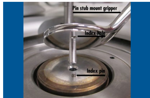
Figure 8. Use the pin stub mount gripper to insert the pin stub mount into the stage. Align the stub index hole with the stage index pin.
