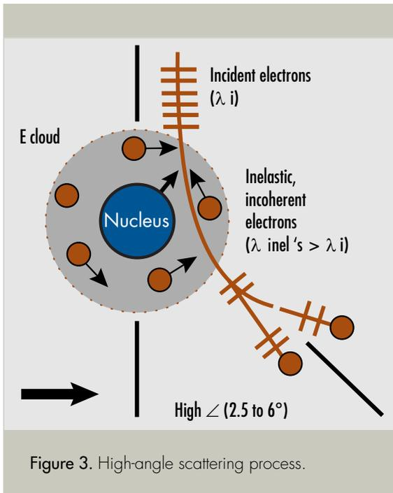
Figure 3. High-angle scattering process.
