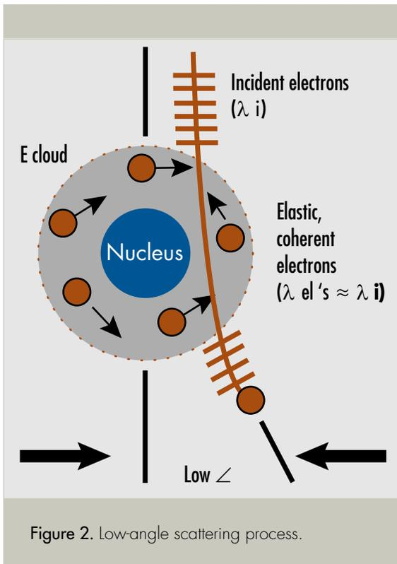
Figure 2. Low-angle scattering process.
