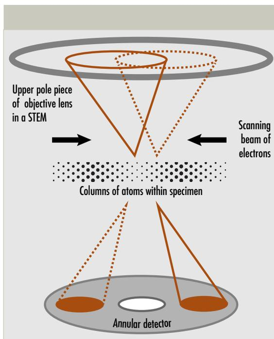
Figure 4. HAADF sampling geometry in a STEM.
